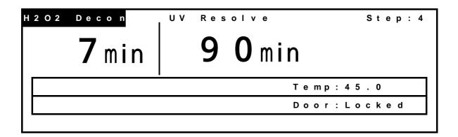
**9.** After completion of  $H_2O_2$  mist generation, "UV Resolve" will flash at the top of the screen, and  $H_2O_2$  gas resolution by UV light will start.
